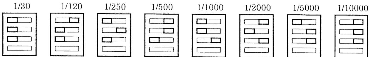
Note: The bottom switch is spare and does not affect the setting.
