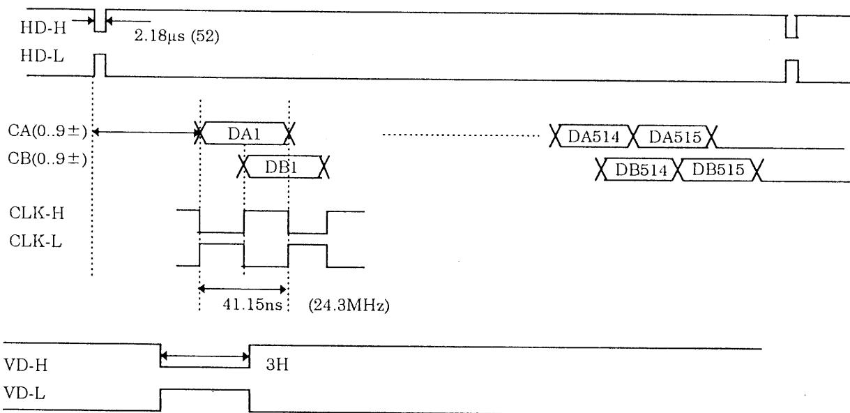
Level: RS-422A rating (High: more than 3.4 V, Low: less than 0.4 V)
