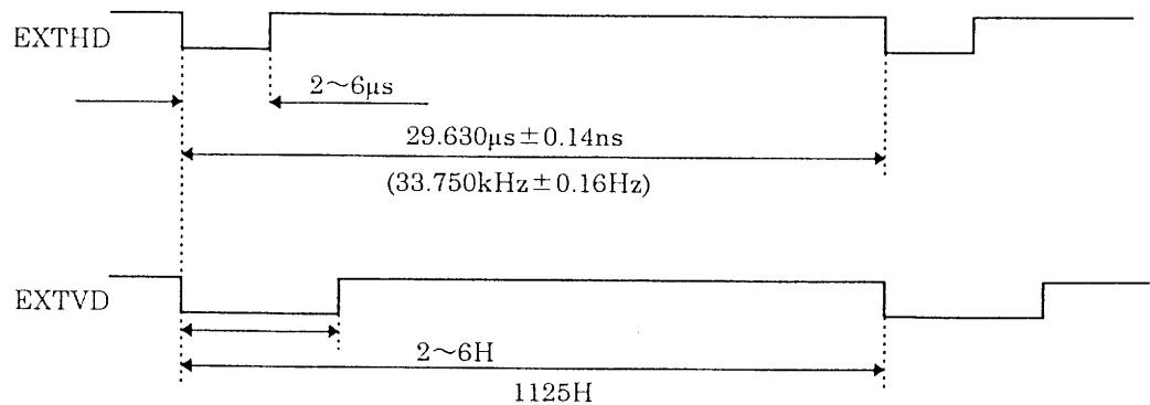
Align falling edges of external HD and VD.
